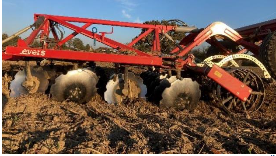
Figure 33: Mechanization for soil cultivation used at the Žnidaričs' farm. Left: circular harrows for soil cultivation. Right: The comb har-row tool for weed control in early stages of cereal growth.
