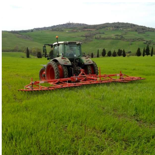
Fig.1 tractor with soft tooth harrow for weed removal in winter wheat
