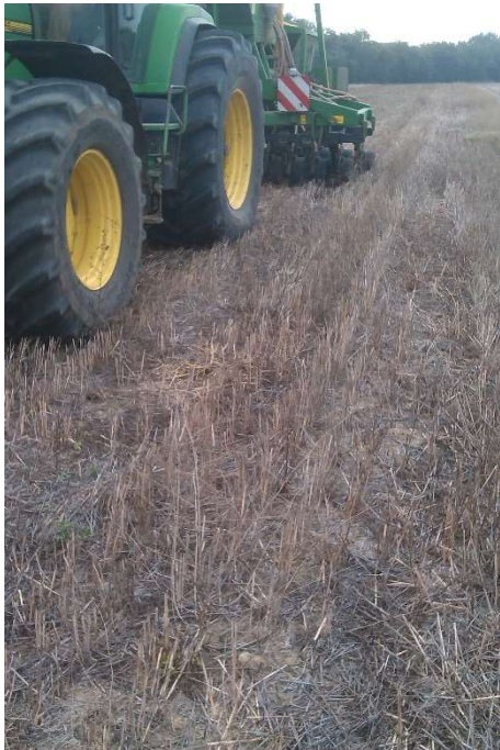
Fig.3 Direct sowing of winter barley in the winter wheat straw of the previous cycle
