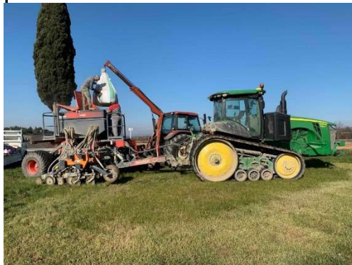
Fig. 1 Sod seeding of winter wheat by means of tractor and sod seeding machine
