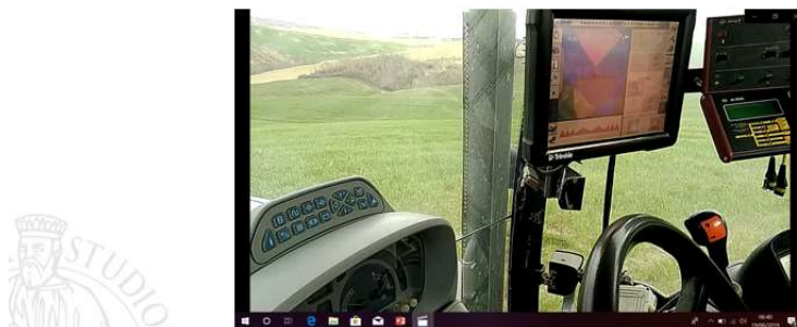
Fig.5 Digital devices for precision fertilization and sowing.
