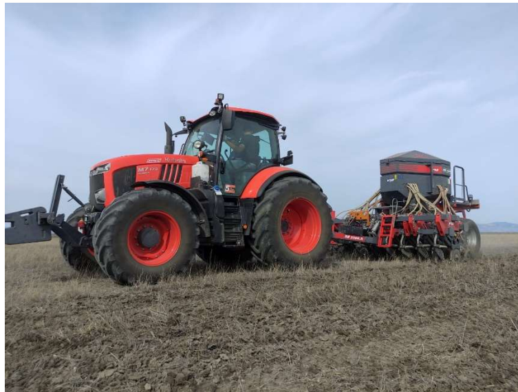
Fig. 2 Sod seeding of winter wheat by means of tractor and sod seeding machine
